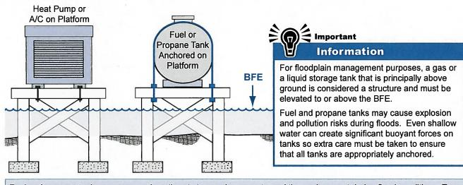
Fuel and propane tanks can pose serious threats to people, property, and the environment during flood conditions. Even shallow water can create a large buoyant force on tanks. Videos on "Fuel Tank Flood Hazards" and "How to Anchor Home Fuel Tanks" are available from FEMA Publications at 1-800-480-2520 and "How-To Guides" on anchoring fuel tanks and other flood damage reduction techniques are available at: http://www.fema.gov/library/viewRecord.do?id=3262.
