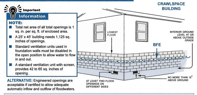
Solid perimeter walls can enclose floodprone areas. A crawlspace is a good way to elevate just a couple of feet. In all cases the following are required: flood openings, utilities elevated to or above the BFE, flood resistant materials and limitations on use of enclosures below the lowest floor. Check with the local permit office for details and restrictions.
