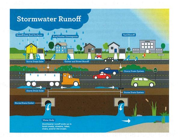
Stormwater is precipitation from either a rain event or snow melt that falls on impervious surfaces, like streets or roofs and eventually flows into storm drains that lead to lakes and rivers.
